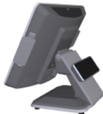
The P1535 also supports extended mounting options for the 2x20 and 10" customer displays as well as a 15" display option. These can be ordered separately. Please see the **Model Accessories** section or the Display Order and Configuration Guide for more information.
